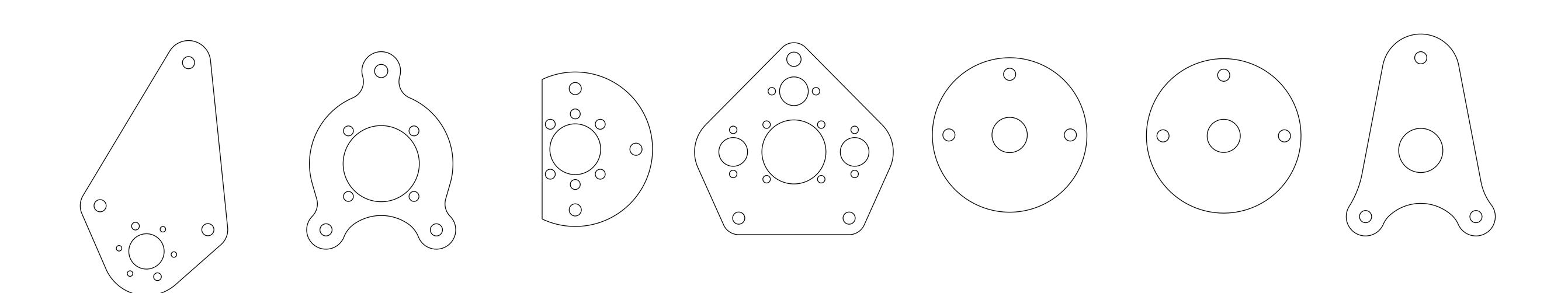
From any 6mm aluminium plate with a minimal RP 0.2 of 150MPA
