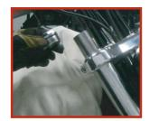
4. With the factory fork caps removed, clean and inspect the threads. Install the RSD fork cap by compressing the fork spring and threading the fork cap clockwise using the large adjustable wrench. Thread the RSD fork cap completely into the fork tube until it bottoms out and tighten securely. Tip: use blue painters tape to protect the fork adjuster during installation. Before installing the RSD fork adjuster cap make sure the adjuster is at the highest position to allow easier installation.
